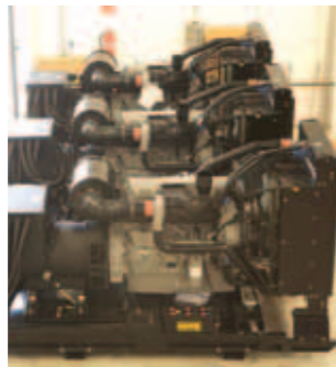
Above right: Himoinsa's HPW400T5 generating set, powered by Perkins' 2306C-E14TAG3, powers the large compactor as it strengthens the ground in Palm Deira.
